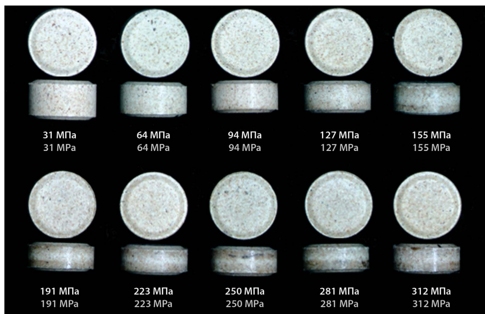
Figure 5. Briquettes of ground Cichorium intybus L. roots (fraction 180–250 μm) obtained at different compression pressures
